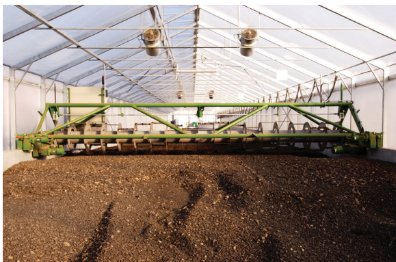
Figure 7: Solar drying in greenhouses (left) and thermal dryer (right). Credit photo: suezwatertechnologies.com
